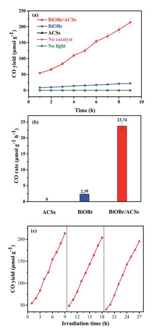
Fig. 6 Photocatalytic  $CO_2$  reduction over BiOBr and BiOBr/ACSs samples under UV-vis irradiation: (a) CO yield, (b) CO rate and (c) cyclic experiments.
