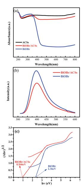
Fig. 4 (a) DRS of the as-prepared samples; (b) PL spectra of BiOBr and BiOBr/ACSs samples; and (c) plots of  $(\alpha h v)^{1/2}$  versus photon energy (hv).
