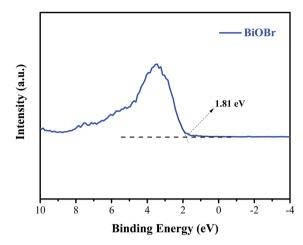
Fig. 7 Valence-band XPS spectra of BiOBr.
