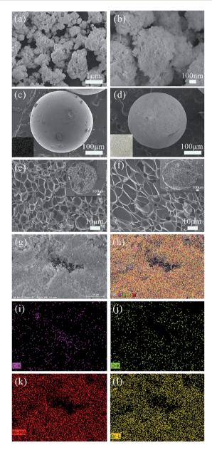
Fig. 2 Low (a) and high (b) magnification SEM images of BiOBr, low-magnification SEM images of ACSs (c) and BiOBr/ACSs (d) (inset c: an image of ACSs; inset d: an image of BiOBr/ACSs), a high-magnification SEM image of ACSs (e) and BiOBr/ACSs (f) cross profiles (inset: low-magnification SEM images of ACSs (e) and BiOBr/ACSs (f) cross profile); (g and h) EDX mappings of the BiOBr/ACSs samples, C (i), O (j), Bi (k), and Br (l) elements.
