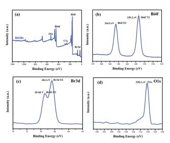
Fig. 3 Survey XPS spectra (a) and high-resolution XPS spectra of BiOBr: Bi 4f (b), Br 3d (c) and O 1s (d).
