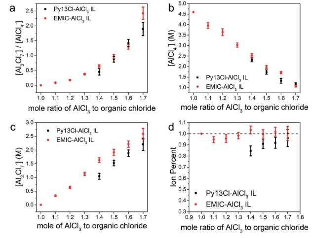
Fig. 4 Species concentrations and ion percent comparison between Py13Cl–AlCl<sub>3</sub> and EMIC-AlCl<sub>3</sub> ionic liquids (a) [Dimer] to [Monomer] ratios comparison between these two ionic liquids, (b) monomer concentration comparison between these two ionic liquids, (c) dimer concentration comparison between these two ionic liquids, (d) ion percent comparison between these two ionic liquids.
