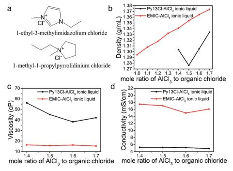
Fig. 1 Structures and physical properties of Py13Cl-AlCl<sub>3</sub> and EMIC-AlCl<sub>3</sub> ionic liquid. (a) The structure of EMIC and Py13Cl, (b) density comparison between Py13Cl-AlCl<sub>3</sub> and EMIC-AlCl<sub>3</sub>, (c) viscosity comparison between Py13Cl-AlCl<sub>3</sub> and EMIC-AlCl<sub>3</sub> measured at 23-24 °C. (d) Conductivity comparison between Py13Cl-AlCl<sub>3</sub> and EMIC-AlCl<sub>3</sub> measured at 25 °C
