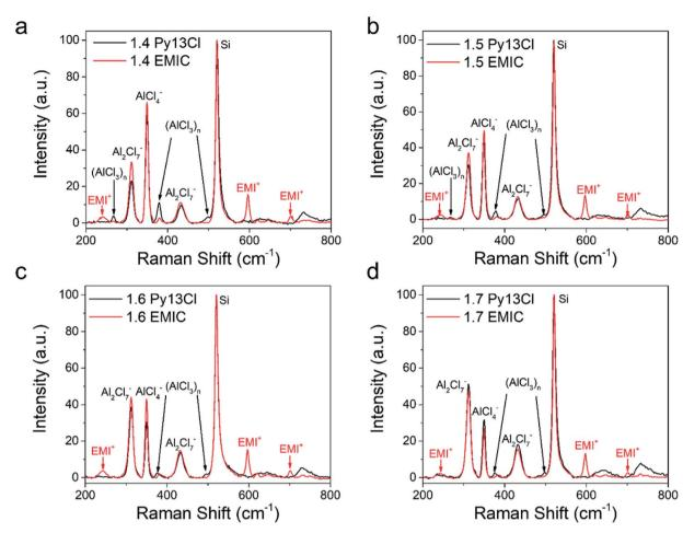
Fig. 3 Raman spectra comparison between Py13Cl-AlCl<sub>3</sub> and EMIC-AlCl<sub>3</sub> ionic liquid. (a) 1.4 Py13Cl and 1.4 EMIC comparison, (b) 1.5 Py13Cl and 1.5 EMIC comparison, (c) 1.6 Py13Cl and 1.6 EMIC comparison, (d) 1.7 Py13Cl and 1.7 EMIC comparison.
