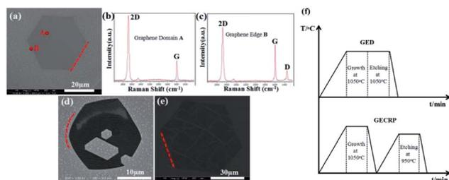
**Fig. 1** (a) SEM image of the synthesized hexagonal graphene domain. (b) and (c) Raman spectra of domain region A and edge B, respectively. (d) SEM image of the graphene domain etched directly after growth. (e) SEM image of the graphene domain etched after cooling and reheating. (f) Simple view of the growth and etching process of the two kinds of samples.
