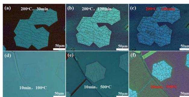
**Fig. 2** Optical microscopy images of graphene domains after etching. (a–c) Degree of etching depending on the etching times of 30, 120, and 240 min, respectively. The etching temperature was 200 °C. (d–f) Degree of etching depending on the etching temperatures of 100, 500, and 950 °C. The etching time was 10 min. The gas flow rate of etching was 2 : 5 (200 sccm  $H_2$  and 500 sccm Ar).
