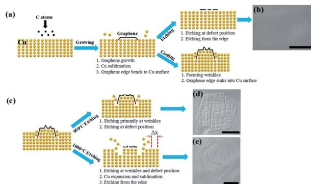
Fig. 5 Schematic of the entire morphological variation of graphene during cooling and etching. (a) Process of graphene growth and direct etching; the graphene edge sinks into the Cu substrate during cooling. (b) Optical microscopy image of GED at 1050 °C. (c) Schematic of the distinction between etching at 950 and 1000 °C. (d and e) Optical microscopy images of GECRP at 950 and 1000 °C. The scale bar is 20  $\mu\text{m}$ .
