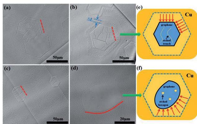
Fig. 3 Optical microscopy images of graphene domains after etching at 1000 °C for (a and b) 10 and (c) 15 min. The gas flow rate of etching was 2 : 50 (20 sccm H<sub>2</sub> and 500 sccm Ar). (d) Optical microscopy image of GED at 1050 °C. (e and f) Schematics of different etching results between GECRP and GED.
