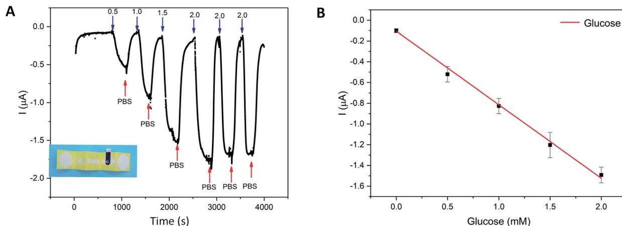
**Fig. 5** Amperometric detection of glucose in the flow injection analysis system with 3D-PMED. (A) Amperometric current response at  $-0.1$  V (vs. Ag/AgCl reference electrode) with alternant injecting of glucose (successive addition of 0.5 mM, 1.0 mM, 1.5 mM, 2.0 mM glucose) and PBS. (B) The calibration plot with the error bar ranging from 0 mM to 2.0 mM.
