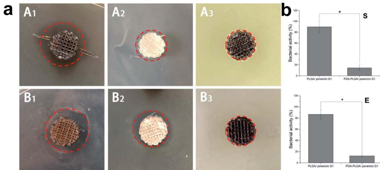
Fig. 8 (a) Inhibition zones study of the PLGA/ponericin G1 (A<sub>2</sub> and B<sub>2</sub>), pDA-PLGA/ponericin G1 (A<sub>1</sub> and B<sub>1</sub>) and pDA-PLGA (A<sub>3</sub> and B<sub>3</sub>) against *E. coli* (E) (B<sub>1</sub>, B<sub>2</sub> and B<sub>3</sub>) and *S. aureus* (S) (A<sub>1</sub>, A<sub>2</sub> and A<sub>3</sub>), (b) relatively antibacterial activity of E and S, after 24 h of culture at 37 °C. ( $n = 3$ ,  $*p < 0.05$ ).
