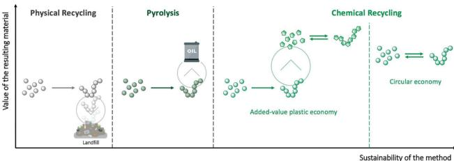
Fig. 1 The different methodologies of polymer recycling.
