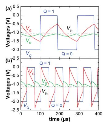
Fig. 2 The measured waveforms in the oscillators in air ambient for  $V_{\rm SS}$  = -2 V,  $R_{\rm S}$  = 1.26 k $\Omega$ , and C = 1 nF. (a) The waveforms in the parabolic oscillator with  $R = 85 \text{ k}\Omega$  resulting in the oscillation frequency  $f_{\text{osc}} =$ 5.3 kHz and duty cycle D = 46%. (b) The waveforms in the bow tie oscillator with  $R = 57 \text{ k}\Omega$ ,  $f_{\text{osc}} = 13.8 \text{ kHz}$ , and D = 55%.
