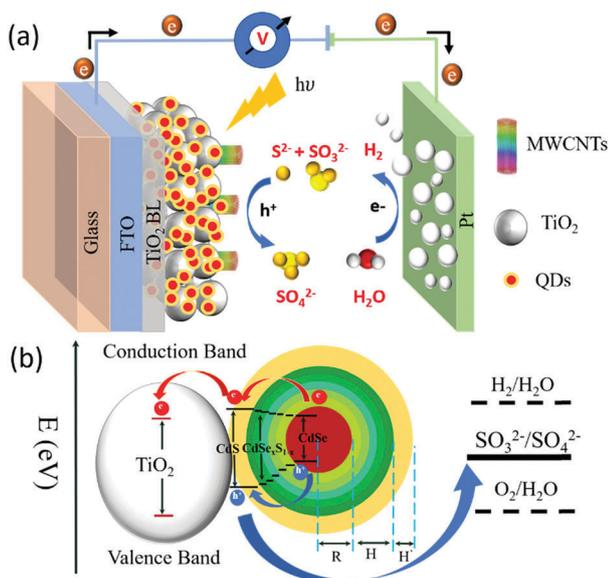
**Fig. 1** Schematic illustration of the: (a) PEC device working principle for  $H_2$  generation; (b) band structure of the graded alloyed core/shell QDs ( $R$  = radius of CdSe core;  $H$  = thickness of the graded alloyed interfacial layers;  $H'$  = thickness of the outer CdS layer) sensitized  $TiO_2$ -MWCNT hybrid film applied as the working electrode. The arrows show the electron and hole transfer process.
