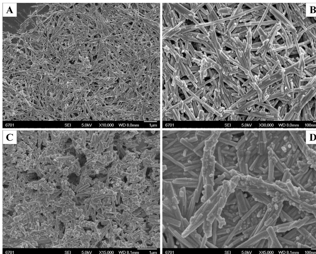
Fig. 2 SEM images: (A and B) CdS nanorods; (C and D) CdS/NiWO<sub>4</sub> (30%).
