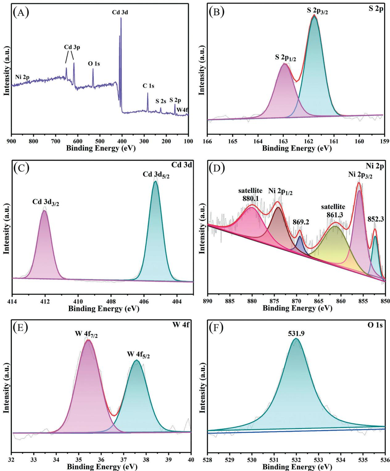
Fig. 4 XPS patterns of the [CdS/NiWO<sub>4</sub> (30%)] sample. (A) Survey, (B) S 2p, (C) Cd 3d, (D) Ni 2p, (E) W 4f and (F) O 1s scan spectra.
