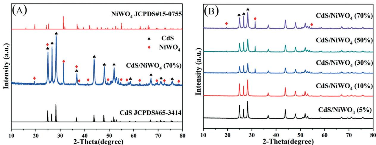
Fig. 1 The XRD patterns of (A) CdS/NiWO<sub>4</sub> (70%) and JCPDS of CdS and NiWO<sub>4</sub>; (B) the XRD patterns of [CdS/NiWO<sub>4</sub> (x%)] ( $x = 5, 10, 30, 50, 70$ ).
