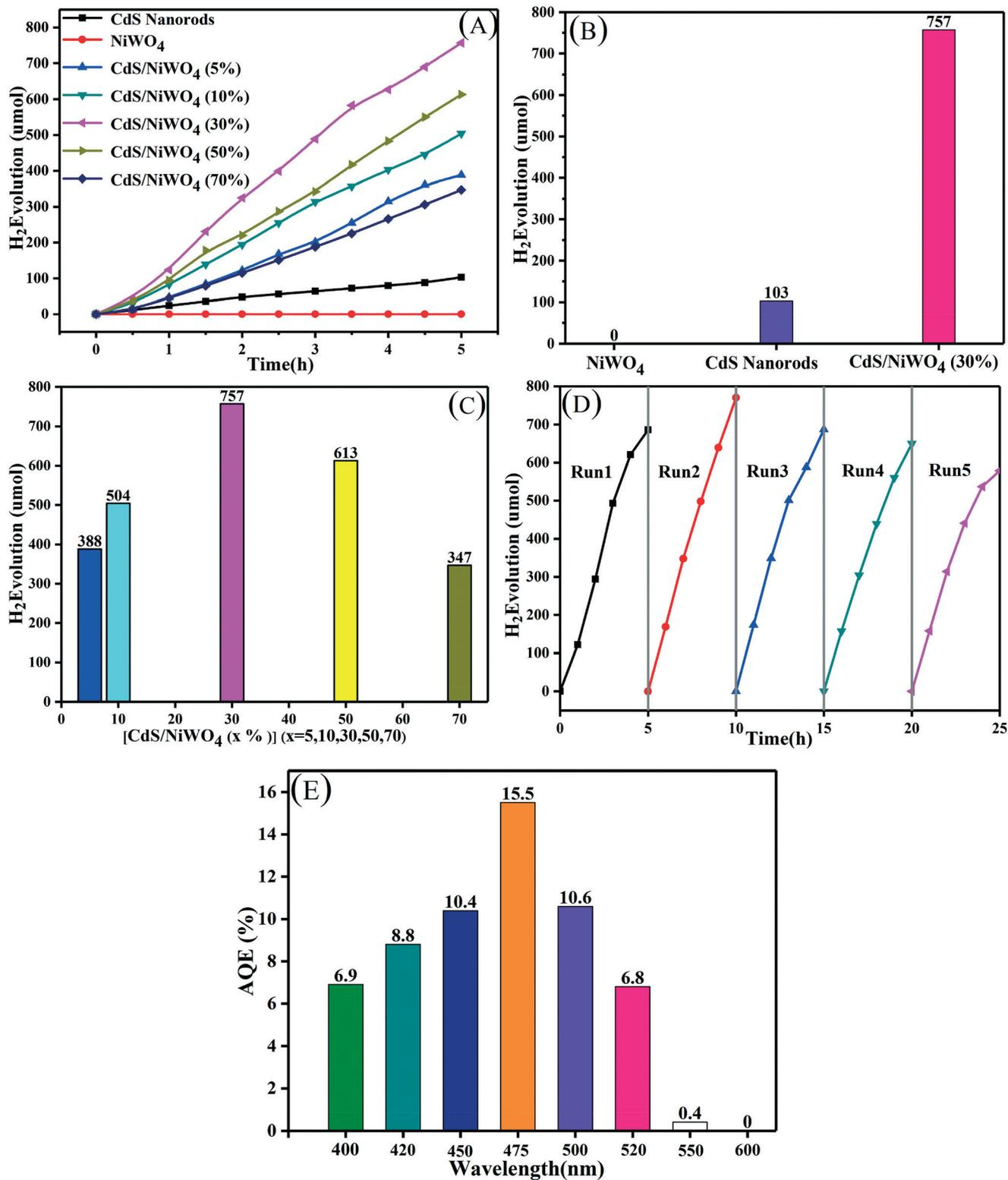
Fig. 7 (A–C) The H<sub>2</sub> production activity curves of CdS nanorods, NiWO<sub>4</sub> and [CdS/NiWO<sub>4</sub> (x%)] (x = 5, 10, 30, 50, 70) in 30 ml 10% lactic acid solution; (D) stability test on the [CdS/NiWO<sub>4</sub> (30%)] sample; (E) the AQE of the [CdS/NiWO<sub>4</sub> (30%)] sample in 30 ml 10% lactic acid solution.
