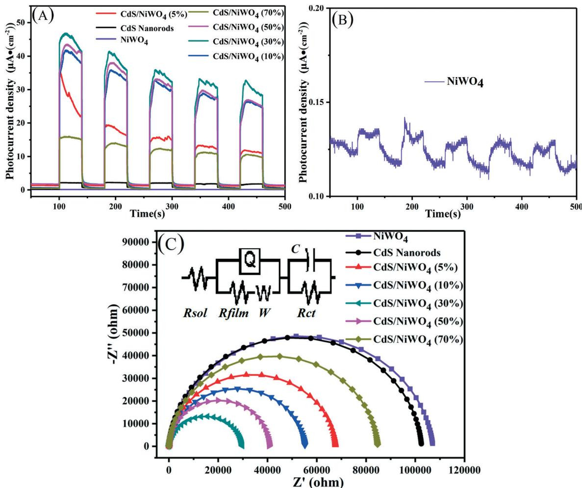
Fig. 9 (A) Transient photocurrent responses; (B) transient photocurrent response of NiWO<sub>4</sub>; (C) electrochemical impedance spectroscopy (EIS) (0.2 M Na<sub>2</sub>SO<sub>4</sub>, λ ≥ 420 nm).
