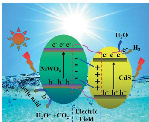
Scheme 1 Photocatalytic mechanism of the CdS/NiWO<sub>4</sub> system.
