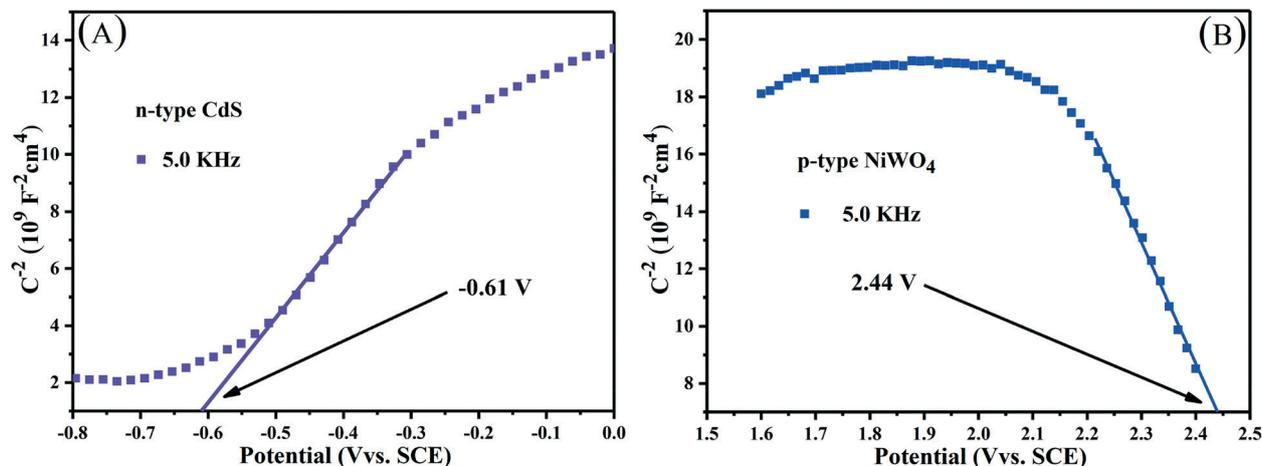
Fig. 10 Mott-Schottky plots of (A) n-type CdS nanorods and (B) p-type NiWO<sub>4</sub> at a frequency of 5.0 kHz.
