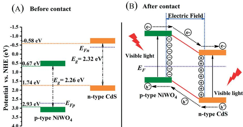
Fig. 11 Schematic diagrams for energy bands of p-NiWO<sub>4</sub> and n-CdS (A) before contact and (B) after the formation of the p-n heterojunction.
