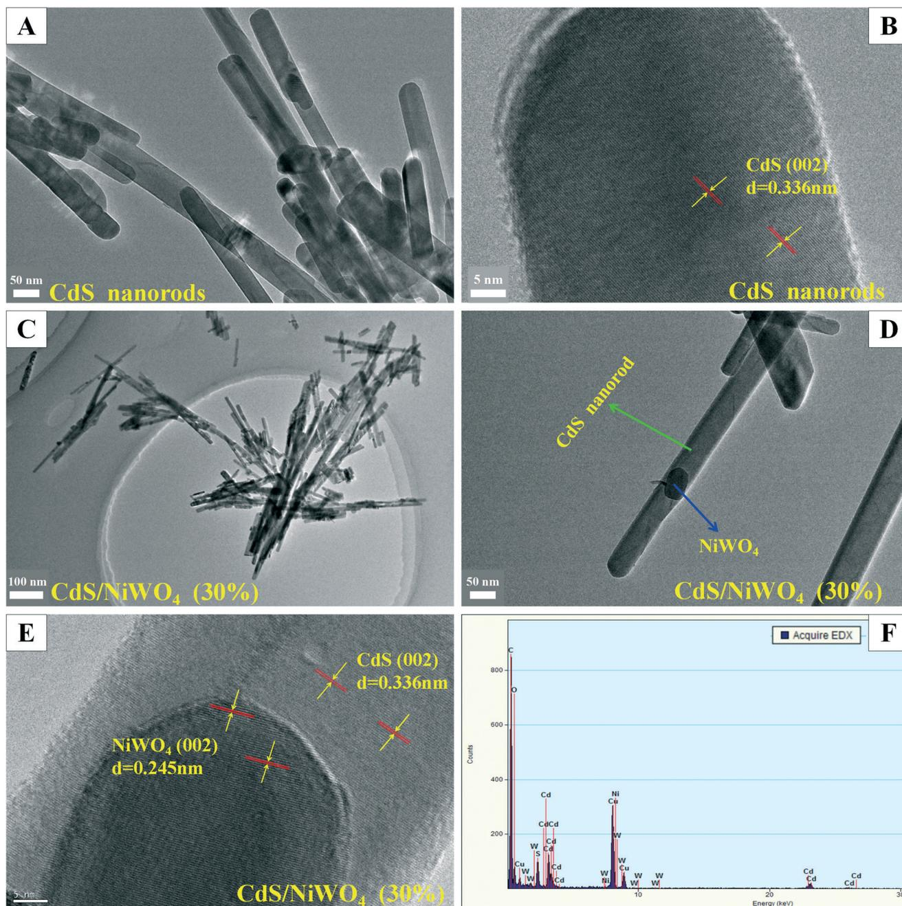
Fig. 3 (A and B) TEM and HRTEM images of CdS nanorods, (C–E) TEM and HRTEM images of [CdS/NiWO<sub>4</sub> (30%)] and (F) EDX spectrum of [CdS/NiWO<sub>4</sub> (30%)].
