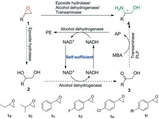
Scheme 1 One-pot asymmetric ring opening of racemic epoxides to enantiopure β-amino alcohols via epoxide hydrolase/alcohol dehydrogenase/transaminase cascade biocatalysis.
