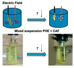
Fig. 10 The experimental arrangement of Li et al. 18 in the presence of an electric field and subsequent cooling crystallisation. Phenazine and caffeine were separately recovered from their suspension in 1,4-dioxane. Reprinted from ref. 18 with permission of Angewandte, Chemie, John Wiley and Sons.
