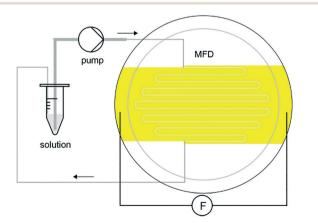
Fig. 6 Continuous flow electric-field assisted crystallization process flow diagrammatic setup of Li and Lakerveld.<sup>54</sup> Reprinted with permission from ref. 54 Copyright (2018) American Chemical Society.
