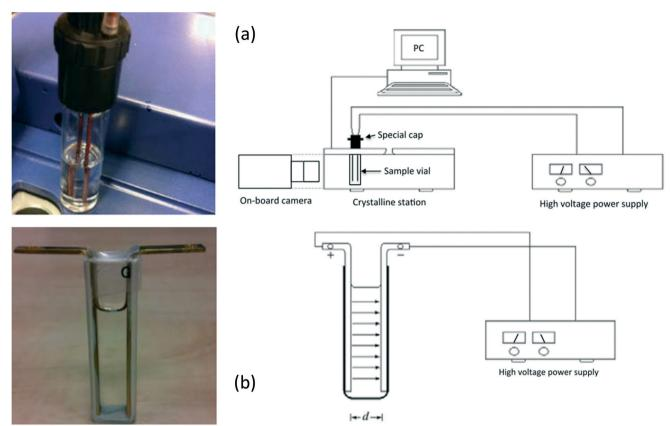
Fig. 8 (a) The parallel-rod arrangement of Radacsi,<sup>59</sup> along with the schematic representation of the scheme and (b) the parallel-plate arrangement with the equivalent schematic. Reprinted with permission from ref. 59.
