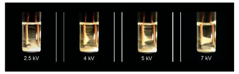
Fig. 9 Experimental observations of Li et al. 18 of particle movement when an inhomogeneous static electric field was applied to a suspension of isonicotinamide in 1,4-dioxane. Reprinted from ref. 18 with permission of Angewandte, Chemie, John Wiley and Sons.
