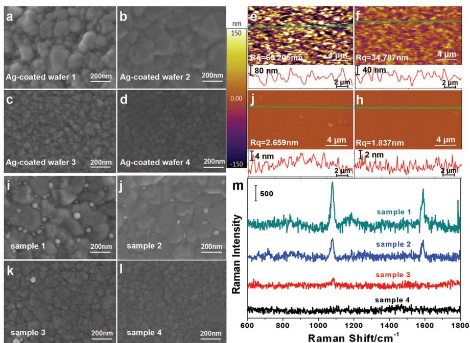
**Fig. 3** (a–d) SEM images of Ag-coated wafers (1–4) fabricated at deposition rates of 0.05, 0.1, 0.2, and 0.4 nm s<sup>-1</sup>, respectively; (e–h) AFM images corresponding to Ag-coated wafers (1–4), and the cross-section profiles marked as the green line are also shown below; (i–l) SEM images of the control samples fabricated using the Ag-coated wafers (1–4), respectively; (m) Raman spectra of the control samples.
