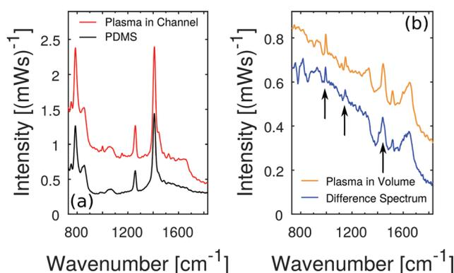
**Fig. 8** NIR Raman spectroscopy of blood plasma in a microfluidic channel with 3 minutes integration time. (a) Fluorescent and Raman scattering from blood plasma are superimposed by the out-of-focus Raman scattering by PDMS. (b) A scaled subtraction of the PDMS Raman signature from the spectrum corrects for the PDMS background and restores the pure spectrum of blood plasma.
