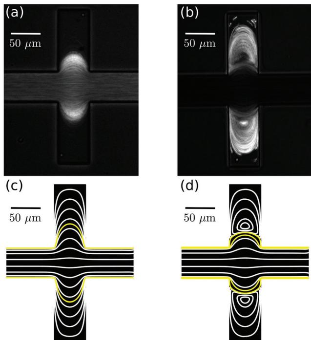
**Fig. 4** Different flow patterns for the same in-plane channel geometry, but different channel depths of  $h = 20 \mu\text{m}$  (a, c) and  $h = 40 \mu\text{m}$  (b, d). Panels (a–b) show the standard deviation of microfluidic experiments whereas panels (c–d) illustrate the streamlines of corresponding creeping flow simulations.
