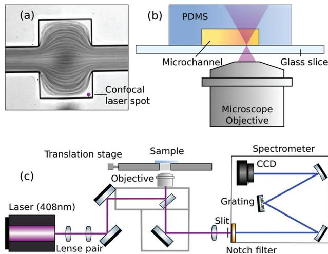
**Fig. 2** Microfluidic Raman setup. (a) The localized cell-free plasma domain in microfluidic whole blood stream is probed by confocal Raman spectroscopy. (b) The Raman laser penetrates both the microfluidic channel and the PDMS host material. (c) The microfluidic chip is mounted on the translation stage of an inverted microscope with confocal laser excitation at 408 nm. Raman emission is analyzed by an imaging dispersive spectrometer.
