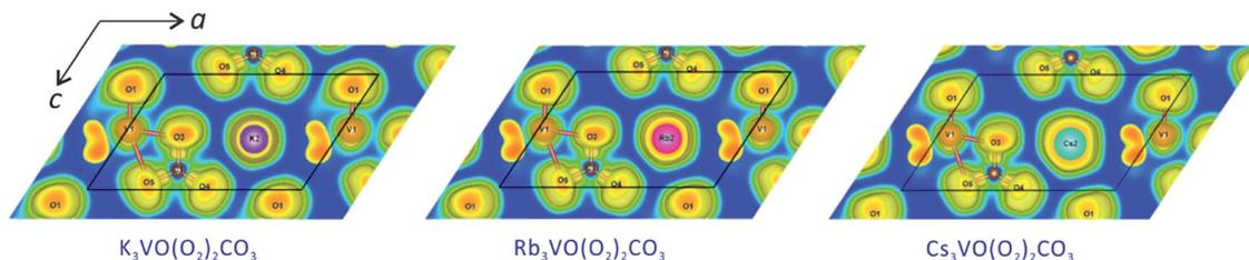
Fig. 5 Three sliced-planes of electron localization function (ELF) of  $A_3VO(O_2)_2CO_3$  ( $A = K, Rb, \text{ and } Cs$ ) in the crystallographic  $ac$ -plane. All diagrams are depicted as filled contour maps. The color scheme ranges from blue to red ( $0-0.7 e^- \text{ per } \text{\AA}^3$ ), and values higher than 0.5 represent the area exceeding the free-electron ELF value. The unit cell is outlined in black.
