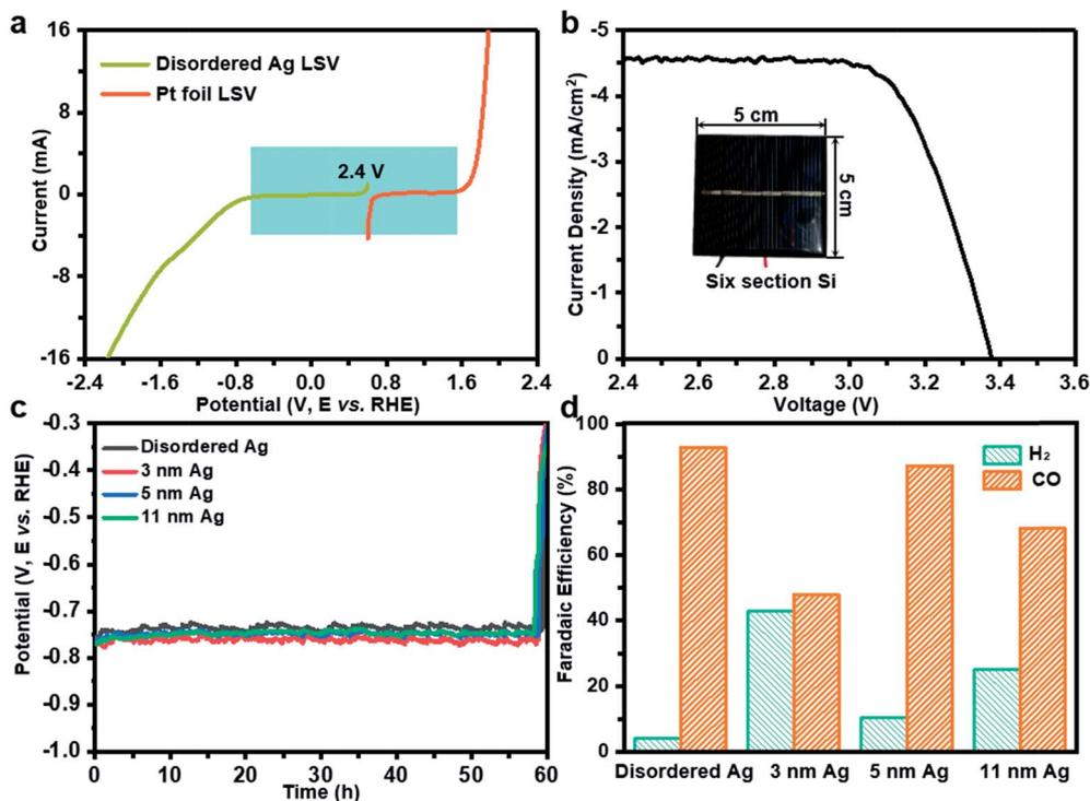
Fig. 3 (a) Performance of the disordered Ag and Pt film towards the CO<sub>2</sub>RR and OER by linear sweep voltammetry at a scan rate of 50 mV s<sup>-1</sup> in 0.1 M KHCO<sub>3</sub>. (b) The current density–voltage characteristics of a six-section a-Si solar cell were measured under AM 1.5G illumination. (c) Cathode voltage and (d) CO FE in the PV-EC system driven by a six-section a-Si solar cell.
