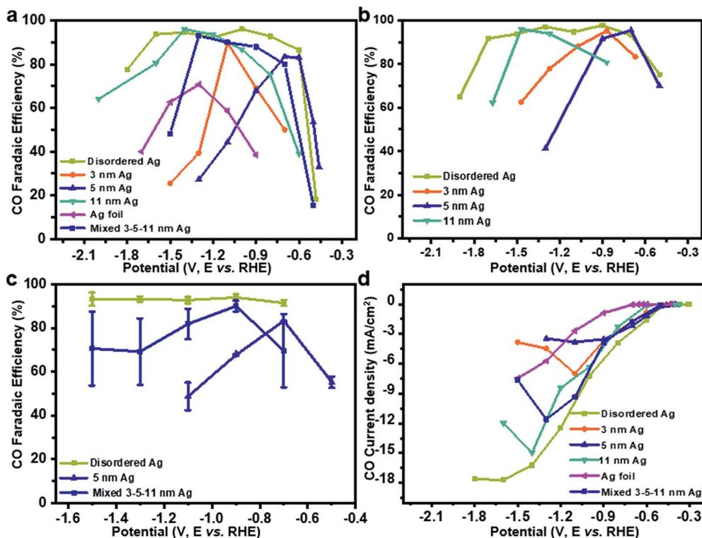
Fig. 2 CO faradaic efficiency depending on applied potential in CO<sub>2</sub> saturated (a) 0.1 M KHCO<sub>3</sub> and (b) 0.1 M KCl, (c) CO faradaic efficiency on a simple mixture of 3–5–11 nm, disordered and 5 nm Ag in 0.1 M KHCO<sub>3</sub> with error bars. (d) CO partial current density depending on applied potential.
