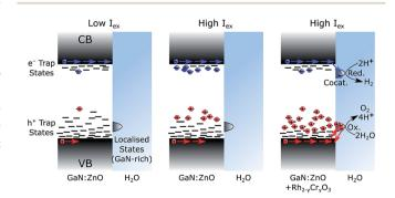
Fig. 7 Schematic representation of trap state filling. The left case shows GaN:ZnO photoexcited with low light flux, the middle case shows GaN:ZnO photoexcited with high light flux, and the right case shows GaN:ZnO/Rh<sub>2-y</sub>Cr<sub>y</sub>O<sub>3</sub> photoexcited with high light flux. Charge distribution reflects a thermalized population, as expected under continuous solar irradiation.
