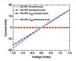
Fig. 3 Current ( $\prime$ ) vs. voltage ( $\prime$ ) plot for pressed pellets of NU-901 and NU-901-C<sub>60</sub>. The scan was performed from -2 V to 2 V and the scan rate was 50 mV s $^{-1}$ .
