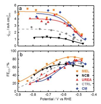
Fig. 4  $CO_2$  reduction data for various Fe-N-C catalysts based on different secondary nitrogen precursors: (a) CO generation rate, (b) faradaic efficiency towards CO production. Experimental conditions:  $CO_2$  saturated 0.1 M KHCO<sub>3</sub>, catalyst loading: 0.75 mg cm<sup>-2</sup> on glassy carbon.
