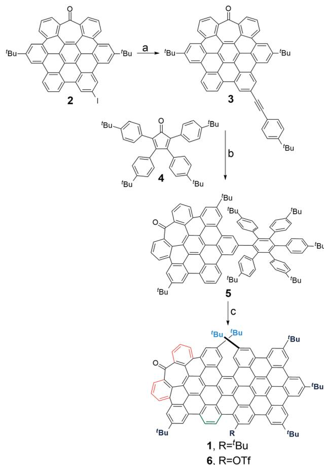
Scheme 1 Synthesis of compound **1**. Reagents and conditions: (a) 4-*tert*-butylphenylacetylene, PdCl<sub>2</sub>(PPh<sub>3</sub>)<sub>2</sub>, CuI, NEt<sub>3</sub>, THF, RT, 16 h, 99%; (b) Ph<sub>2</sub>O, reflux, 8 h, 34%; (c) DDQ, CF<sub>3</sub>SO<sub>3</sub>H, CH<sub>2</sub>Cl<sub>2</sub>, 0 °C, 10 min, **1** (46%) and **6** (5%).
