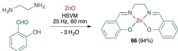
Scheme 46 Mechanochemical synthesis of a zinc–salen complex.
