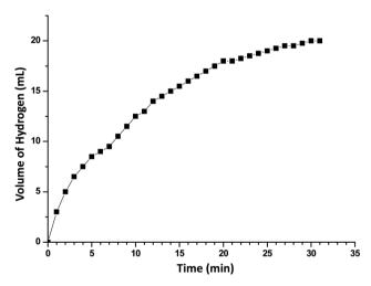
Fig. 4 A representative plot for the volume of  $H_2$  generated from ammonia borane ethanolysis as a function of reaction time in the presence of  $\text{Cu}_2\text{O}$  rhombic dodecahedra. Reaction conditions: catalyst = 4 mg, amount of ammonia borane used = 0.0123 g, temperature = 30 °C. The volume of hydrogen evolved is 20 mL in 31 min.
