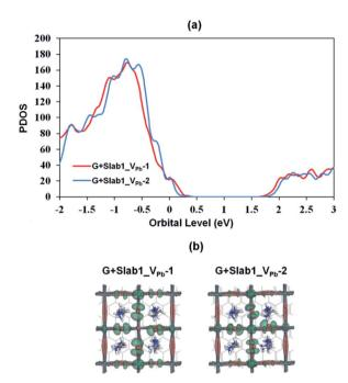
Fig. 13 (a) Calculated partial density of states (PDOS) of MAPbI<sub>3</sub> in the  $V_{Pb}$ -containing graphene + MAPbI<sub>3</sub> hybrids, and (b) the orbital shape of the valence band edges of MAPbI<sub>3</sub> (isovalue: 0.015 a.u.).
