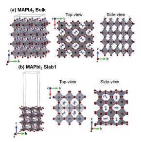
Fig. 1 (a) Bulk and (b) slab  $\mathsf{MAPbI}_3$  models adopted in the present study.
