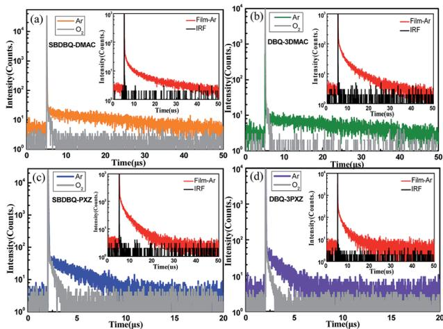
Fig. 3 Transient PL characteristics of (a) SBDBQ-DMAC, (b) DBQ-3DMAC, (c) SBDBQ-PXZ, and (d) DBQ-3PXZ in toluene ( $10^{-5}$  M) under oxygen and argon at room temperature. The insets show the transient PL decay of the corresponding compound in film.
