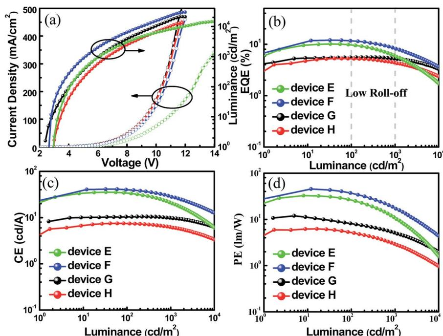
Fig. 6 (a) Current density–voltage–brightness characteristics, (b) EQE versus luminance curves, (c) current efficiency versus luminance curves, and (d) power efficiency versus luminance curves of the non-doped devices (E–H).
