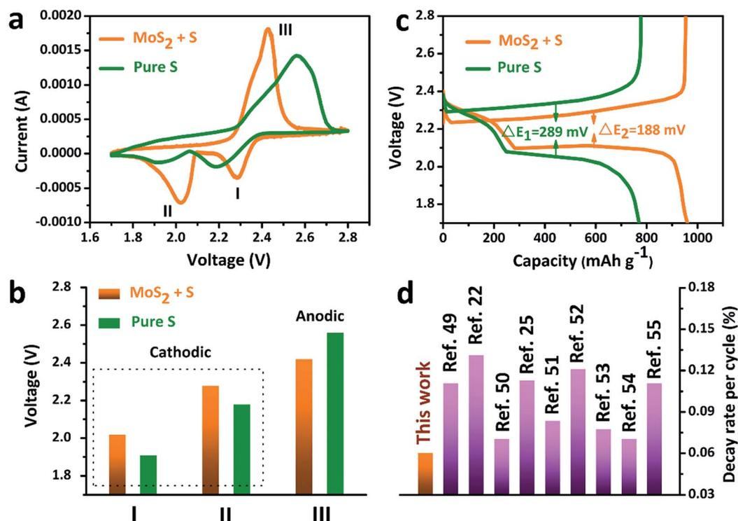
Fig. 5 (a) CV curves, (b) discharge–charge curves and (c) the comparison of the peak voltages of the pure S and MoS<sub>2</sub> + S electrodes. (d) A comparison of the decay rate per cycle with that of other Li–S cathode materials reported in the literature recently.
