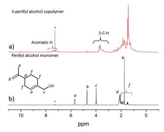
Fig. 2 <sup>1</sup>H NMR for both the sulfur–perillyl alcohol 50: 50 copolymer (a) and the perillyl alcohol monomer (b). Loss of vinylic proton resonances indicate a successful crosslinking by addition across the double bonds, though some aromatic H environments are detected, suggesting some possible hydrogen abstraction. The formation of new peaks in the 3.5–4 ppm region is consistent with the formation of C–S bonds. \* = chloroform.
