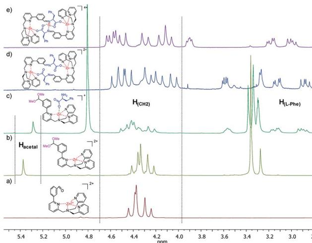
Fig. 2 Comparison of the <sup>1</sup>H-NMR signals for the compounds **1**, **4**, **5-L-Phe**, **1-L-Phe** and **2-L-Phe** in D<sub>3</sub>-acetonitrile. In this region acetal (5.4 to 5.2 ppm), CH<sub>2</sub> picolil (4.6 to 3.9 ppm) and amino acid (3.8 to 2.7 ppm) proton signals are present. The counteranions are perchlorate.
