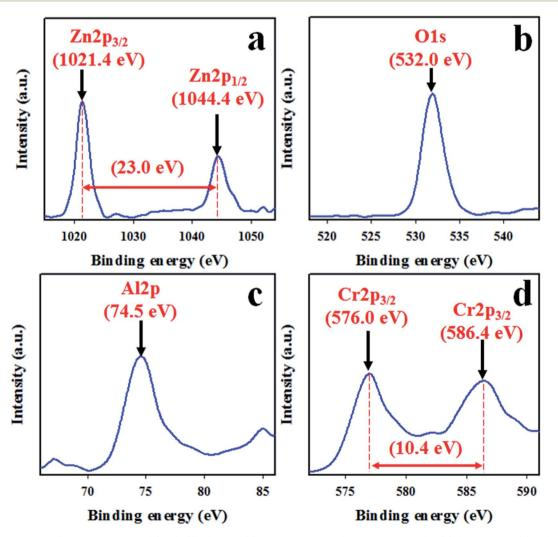
Fig. 2 High resolution XPS spectra of the ZnO/Al<sub>2</sub>O<sub>3</sub>/Cr<sub>2</sub>O<sub>3</sub> NPs. (a) The core level XPS spectrum of Zn 2p, (b) O 1s orbitals, (c) Al 2p orbitals, and (d) the 3/2 spin orbitals of Cr 2p.
