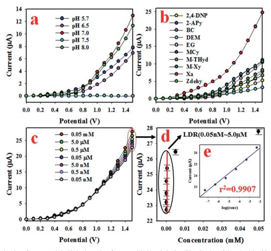
Fig. 4 The estimation of sensor analytical behavior and performance. (a) pH optimization, (b) estimation of the selectivity, (c) concentration variation from lower to higher range, and (d) the calibration curve [inset log(conc.) vs. current].
