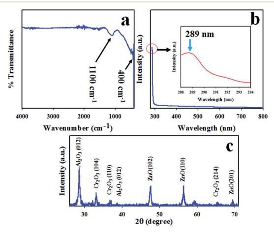
Fig. 1 The optical properties and crystallinity of the synthesized  $ZnO/Al_2O_3/Cr_2O_3$  NPs. (a) FTIR analysis, (b) UV-vis spectrum, and (c) phase crystallinity.
