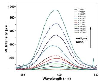
Fig. 6 Sensitivity of the developed FRET-based aptasensor platform against various aflatoxin B1 concentrations (0.002 to 0.2  $\mu$ g  $\mu$ l<sup>-1</sup>).
