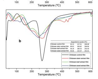
Fig. 2 (a) TGA and (b) DTG thermograms of the chitosan control film and blend films incorporated with *Pistacia terebinthus*' extracts as; chitosan-stem film, chitosan-leaf film and chitosan-seed film.
