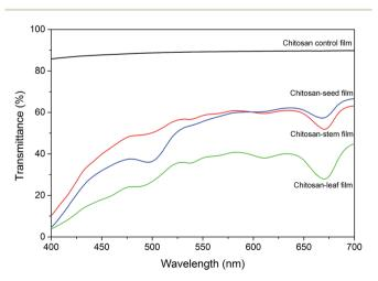
Fig. 6 Optical transmittance of the chitosan control film and blend films incorporated with *Pistacia terebinthus*' extracts as; chitosan-stem film, chitosan-leaf film and chitosan-seed film.
