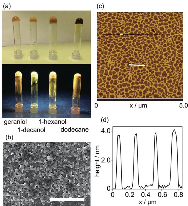
**Fig. 3** (a) Photographs of organogels of **1** (top) under daylight and (bottom) under UV light. (b) The FE-SEM image of the xerogel of **1**. Scale bar displays are 20 μm. (c) The AFM image of **1**. (d) The height profile of the white line in (c).
