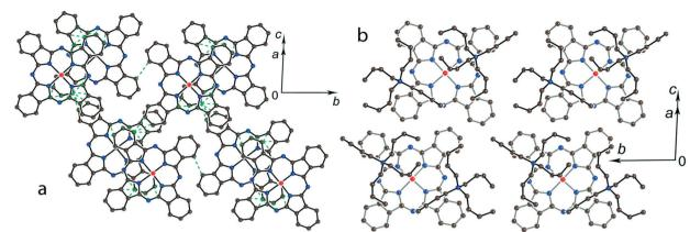
Fig. 3 (a) View of the phthalocyanine layer composed of the  $\pi$ -stacking [{Ti<sup>VO</sup>(Pc<sup>-3-</sup>)}<sup>-1</sup>]<sub>2</sub> dimers in 2.<sup>12</sup> Short van der Waals C,N···C,N contacts are shown by green dashed lines. (b) Projection of the Bu<sub>4</sub>N<sup>+</sup> layer on the phthalocyanine layer. Only one phthalocyanine from the dimer is shown (bonds are shown in grey).
