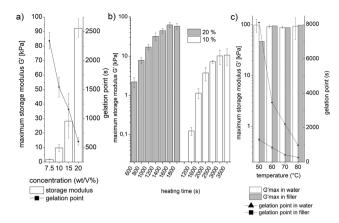
Fig. 2 Hydrogel characterization (maximum G' and gelation point) (procedures and detailed conditions are listed in the ESI†). (a) Variation of sPEG concentration for heating at 60 °C. (b) the effect of different heating times at 60 °C for both 10 and 20 wt/V%, (c) gelation at different temperatures for both water and non-volatile PEG filler as a dispersing agent (20 wt/V% reactive sPEG); measurements are reproduced three times except for 2c with the filler due to long gelation times.
