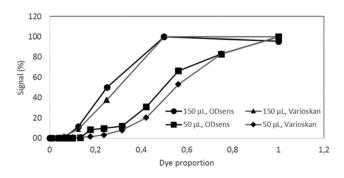
Fig. 4 Validation of the OD sensor – comparison with a Varioskan(R) instrument in 150 and 50  $\mu$ L of sample dilutions of the green food dye (E143), N=3.
