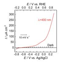
Fig. 7 Current–potential curves of the  $CoO_x/TaON$  photoanode under continuous visible-light irradiation ( $\lambda_{ex} > 400$  nm) and under dark conditions. A 50 mM aqueous solution of NaHCO<sub>3</sub> (pH 6.6) saturated with CO<sub>2</sub> was used as the electrolyte.
