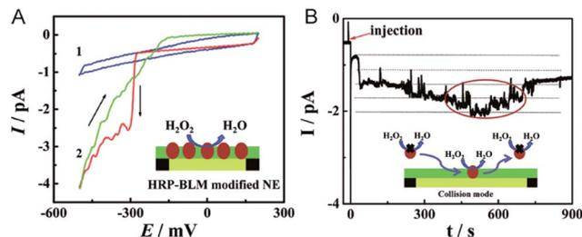
Fig. 5 Studying the single HRP with a BLM-Au nanoelectrode.<sup>6</sup> (A) Cyclic voltammograms of the BLM-Au nanoelectrode (1) and HRP-embedded BLM-Au nanoelectrode (2) in a solution of 20 mM H<sub>2</sub>O<sub>2</sub> and PBS buffer (pH: 7.4). (B) Chronoamperometric response of HRP collision into the BLM-Au electrode.<sup>6</sup> Reproduced by permission of ref. 6 from The Royal Society of Chemistry.
