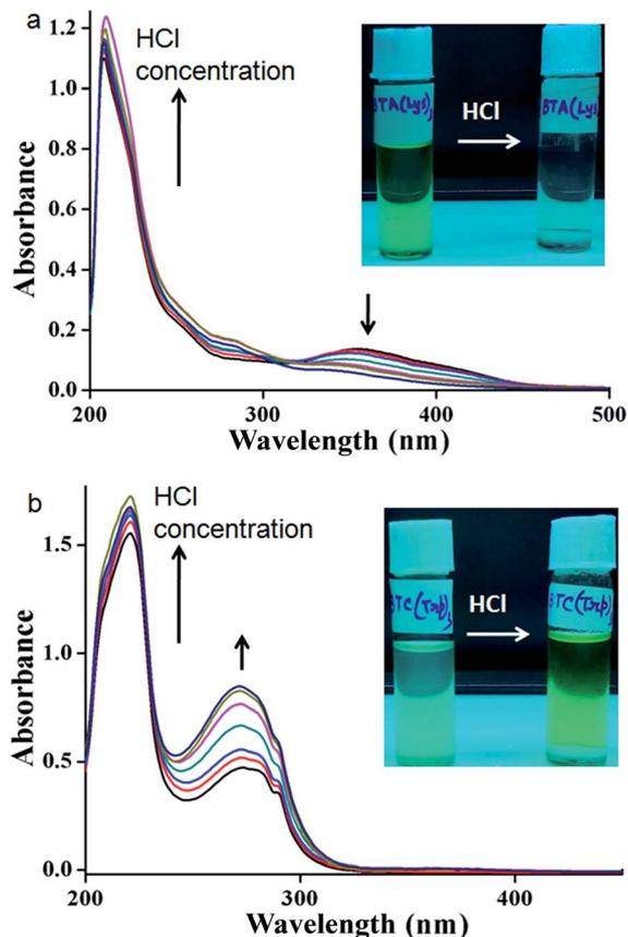
Fig. 2 The UV-Vis titration of (a) trisamide 1 and (b) trisamide 2 methanol solution ( $1.984 \times 10^{-4}$  M) and ( $3.451 \times 10^{-5}$  M) respectively with gradual addition of 0.12 M HCl. Inset: colour change by addition of HCl.
