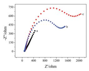
Fig. 2 EIS of 10.00 mM  $[Fe(CN)_6]^{3-/4-}$  containing 0.1 M KCl on the different electrodes. (a) GCE, (b) AuNPs-cPC-cDNA/GCE and (c) apt/AuNPs-cPC-cDNA/GCE.
