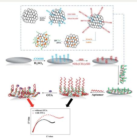
Scheme 1 Schematic illustration of fabrication of the apt/AuNPs-cPC-cDNA/GCE sensor and its application for OTA detection.
