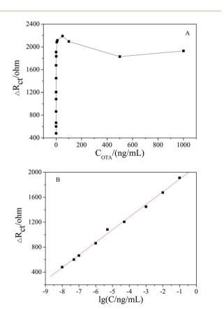
Fig. 6 (A) EIS of apt/AuNPs-cPC-cDNA/GCE with OTA concentration in the range of 1  $\times$  10 $^{-8}$  to 1000 ng mL $^{-1}$ . (B) Linear relationship curve between  $\Delta R_{\rm ct}$  and Ig[OTA].
