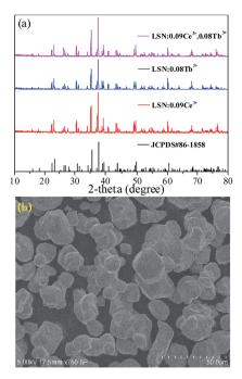
Fig. 1 (a) Powder XRD patterns of  $La_{0.91}Si_3N_5:0.09Ce^{3+}$ ,  $La_{0.92}Si_3-N_5:0.08Tb^{3+}$  and  $La_{0.83}Si_3N_5:0.09Ce^{3+}$ ,0.08Tb<sup>3+</sup> phosphors. The standard data of CeSi $_3N_5$  (JCPDS No. 86-1858) is show as a reference. (b) SEM image of the as-prepared  $La_{0.83}Si_3N_5:0.09Ce^{3+}$ ,0.08Tb<sup>3+</sup> phosphor.
