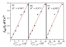
Fig. 9 Dependence of  $I_{SO}/I_S$  of Ce<sup>3+</sup> on (a) C<sup>6/3</sup>, (b) C<sup>8/3</sup> and (c) C<sup>10/3</sup>. The red lines indicate the fitting behaviors.
