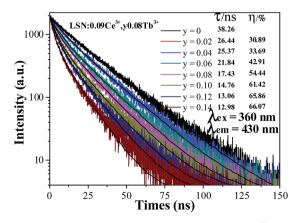
Fig. 8 Decay curves for the luminescence of  $Ce^{3+}$  ions in LSN:0.09 $Ce^{3+}$ ,yTb $^{3+}$  phosphors (excited at 360 nm, monitored at 430 nm).
