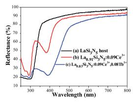
Fig. 6 Reflectance spectra of LaSi<sub>3</sub>N<sub>5</sub> host (a), La<sub>0.91</sub>Si<sub>3</sub>N<sub>5</sub>:0.09Ce<sup>3+</sup> (b), and La<sub>0.83</sub>Si<sub>3</sub>N<sub>5</sub>:0.09Ce<sup>3+</sup>,0.08Tb<sup>3+</sup> (c).
