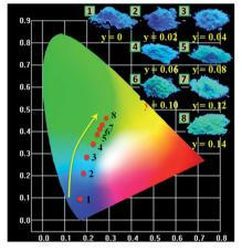
Fig. 11 CIE chromaticity coordinates diagram of LSN: $0.09Ce^{3+}$ , $yTb^{3+}$  (y = 0, 0.02, 0.04, 0.06, 0.08, 0.10, 0.12, 0.14) (point no. 1-8) and the digital photographs of corresponding samples under 365 nm UV lamp.
