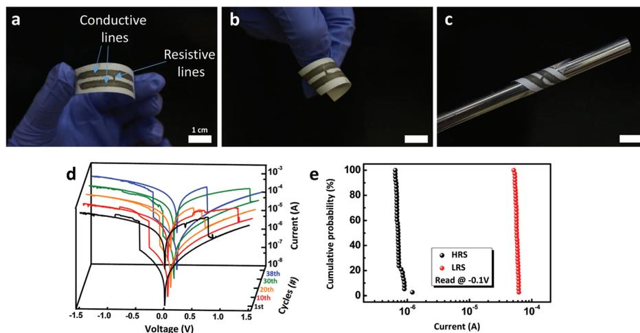
**Fig. 6** Resistive switching memory devices fabricated by pencil writing. (a–c) The optical images of pencil-drawn memory devices on papers (Scale bar: 1 cm). Memory devices are fabricated on papers, so folding, bending, or wrapping can be done. (d)  $I$ – $V$  characteristics of the memory device on paper. (e) Cumulative probability of high resistance state (HRS) and low resistance state (LRS) current through 38 cycles.
