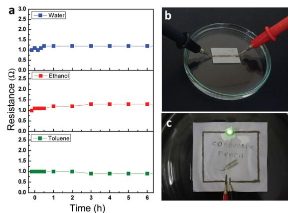
**Fig. 5** Stability of drawn conductive lines on copy paper under wet conditions. (a) Resistance change according to time under various chemical solvent wetting; in DI water (blue), ethanol (red), and toluene (green). (b) The optical image of the measured configuration. The paper with a drawn conductive line is completely soaked in water, ethanol, or toluene in the glass petri dish. (c) The optical image of LED lighting with a hybrid pencil drawn conductive line under water wetting.
