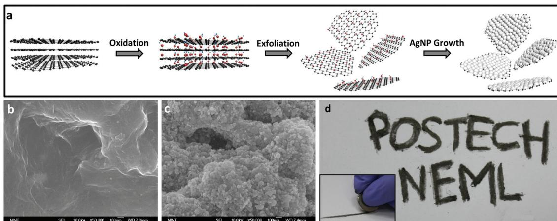
**Fig. 1** (a) Schematic images depicting the procedure of fabricating conductive AgNPs/rGO hybrid powder. SEM images of (b) pure rGO and (c) synthesized AgNPs/rGO hybrid powders. (d) Letters drawn with the AgNPs/rGO pellet. Inset shows a drawing process.
