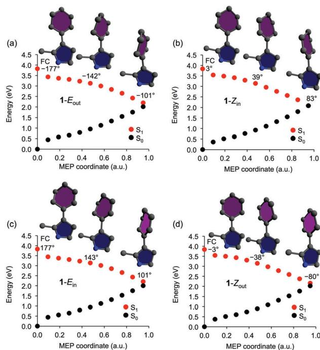
**Fig. 1** Minimum energy paths (MEPs) from the  $S_1$  Franck–Condon (FC) points of the  $E_{\text{out}}$  (a),  $Z_{\text{in}}$  (b),  $E_{\text{in}}$  (c) and  $Z_{\text{out}}$  (d) isomers of motor **1**. Shown are also the molecular geometries at the FC point and at two additional points along the paths, as well as the corresponding  $\omega$  dihedral angles.
