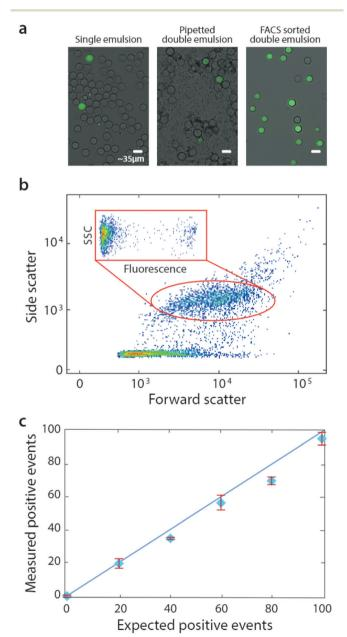
Fig. 3 Bulk dispersal allows accurate droplet quantitation over a range of concentrations. Microfluidic droplets are generated (a, left) and bulk double emulsified into aqueous carrier via pipetting (a, middle), followed by analysis and sorting with flow cytometry (a, right). During FACS, scattering and fluorescence are measured (b). The number of detected positive droplets scales with the number of positives added to the single emulsion (c).
