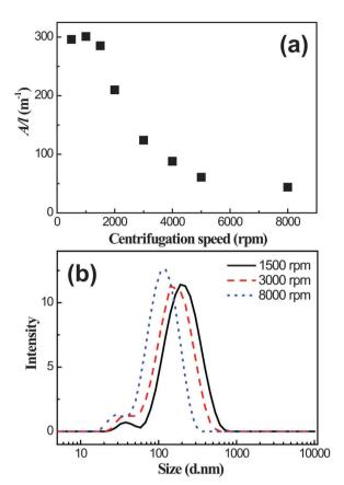
Fig. 4 (a) The A/l values at 660 nm for the  $I_3C-CI_3$ -treated graphene dispersions after centrifugation at different speeds for 90 min. (b) Size distributions of the dispersed graphene flakes in solutions centrifuged at different speeds as measured by DLS.
