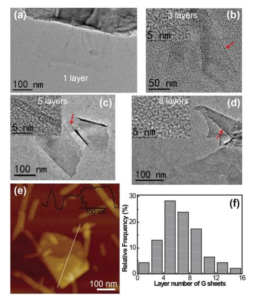
Fig. 6 TEM images of (a) a single-layer graphene sheet, (b) a tri-layer graphene sheet, (c) a five-layer graphene sheet, and (d) an eight-layer graphene sheet. (e) AFM image of a graphene sheet by drop casting onto freshly cleaved mica. (f) Statistical analysis of flake size. Histograms showing flake thickness, expressed as the number of graphene monolayers per flake.
