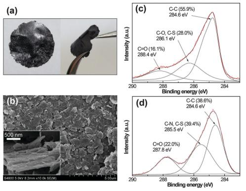
Fig. 8 (a) The photographs and (b) the SEM images (inset, a magnified image) of the graphene/I<sub>3</sub>C-CI<sub>3</sub> composite film prepared by simple filtration of a dispersion through a nylon filter membrane of 0.22 µm pore size. Note that the dispersion was obtained by centrifugation at 5000 rpm for 10 min. XPS profiles (C1s spectra) of (c) the graphene/ $I_3C-CI_3$  composite and (d) the  $I_3C-CI_3$  powder.
