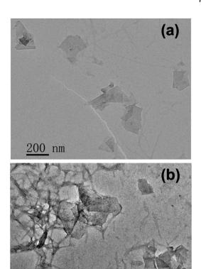
Fig. 5 TEM images of (a) the unstained and (b) the negatively stained samples showing the suspended flake species in the I<sub>3</sub>C-CI<sub>3</sub>-treated graphene dispersion after centrifugation at 5000 rpm for 10 min.
