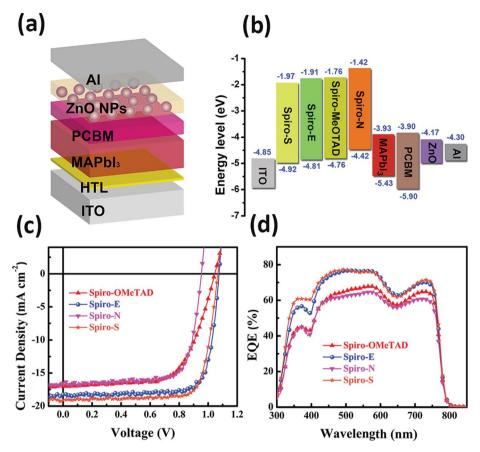
Fig. 3 (a) The structure of the perovskite solar cell devices; (b) energy level diagram of the tested HTMs; (c) photocurrent density–voltage (J-V) curves and (d) EQE spectra of the corresponding solar cells.
