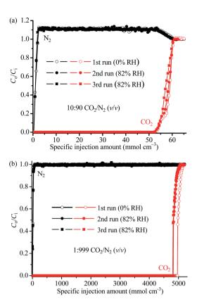
Fig. 5 Repeated breakthrough curves of the 1a column operated at 1 bar. (a)  $10:90 \ \text{CO}_2/\text{N}_2$  (v/v) at  $313 \ \text{K}$ . (b)  $1:999 \ \text{CO}_2/\text{N}_2$  (v/v) mixture at 298 K. Lines are drawn to guide eyes.  $C_i$  and  $C_o$  are the concentrations of each gas at the inlet and outlet, respectively.
