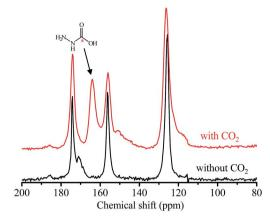
Fig. 3 Solid-state  $^{13}$ C NMR spectra of **1a** with and without adsorbed CO<sub>2</sub>. An asterisk (\*) marks the carbon atom of CO<sub>2</sub>.
