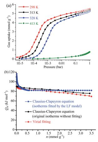
Fig. 2 (a)  $CO_2$  adsorption (solid) and desorption (open) isotherms measured at 298, 313, 328 and 413 K and (b) the coverage-dependent  $CO_2$  adsorption enthalpy of 1a.
