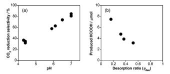
Fig. 4 (a) Selectivity of  $CO_2$  reduction ( $sel_{CO_2}$ ) vs. pH of the reaction solution in the photocatalytic reactions. (b) Produced amount of HCOOH vs. desorption ratio of RuRu ( $\eta_{des}$ ) by the photocatalytic reactions with various concentration of NaH<sub>2</sub>PO<sub>4</sub> (pH = 4.4).
