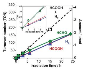
Fig. 6 Time courses of HCOOH (red), H<sub>2</sub> (blue) and HCHO (green) formation along with the sum of HCOOH and H<sub>2</sub> (black broken line) in the photocatalytic reaction: RuRu/Ag/TaON (4 mg) in a H<sub>2</sub>O–MeOH (4 : 1 v/v) mixed solution (4 mL) was irradiated by visible light ( $\lambda$  > 400 nm) under a CO<sub>2</sub> atmosphere. Inset shows enlarged time courses until 4 h irradiation.
