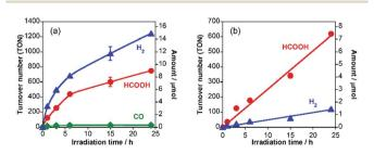
Fig. 2 Time courses of HCOOH (red),  $H_2$  (blue) and CO (green) formation by visible-light ( $\lambda$  > 400 nm) irradiation to RuRu/Ag/TaON (4 mg) in EDTA·2Na (10 mM) aqueous solution (4 mL) without (a) and with (b) Na<sub>2</sub>CO<sub>3</sub> (0.1 M) under a CO<sub>2</sub> atmosphere.
