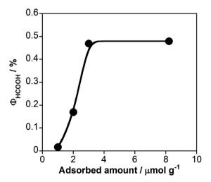
Fig. 5 Relationship between  $\Phi_{\rm HCOOH}$  and loading amount of RuRu in the photocatalytic reaction using RuRu/Ag/TaON (30 mg) and EDTA·2Na (10 mM) in aqueous solution (10 mL) with 400 nm monochromatic light irradiation under a CO<sub>2</sub> atmosphere.
