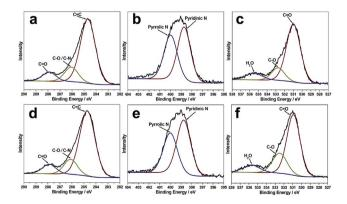
Fig. 2 The C 1s, N 1s and O 1s XPS spectra for the R-CNDs (a–c) and B-CNDs (d–f).
