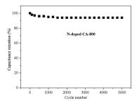
Fig. 9 The cycling stability of N-doped CA-800 at a current density of 1.0 A  $\rm g^{-1}.$
