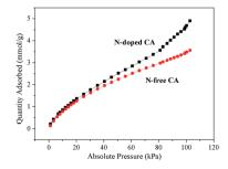
Fig. 6  $CO_2$  adsorption isotherms of N-free CA-800 and N-doped CA-800.
