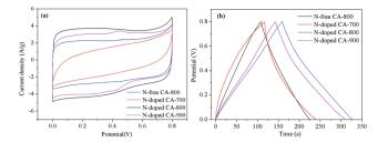
Fig. 7 CV curves at 20 mV s $^{-1}$  (a) and galvanostatic charge/discharge curves at 1.0 A g $^{-1}$  (b) of carbon aerogels.
