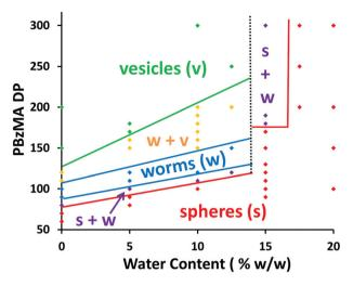
Fig. 5 Phase diagram showing the morphology obtained for PDMA $_{43}$ - PBzMA $_x$  diblock copolymers synthesized via RAFT dispersion polymerization of BzMA at 70 °C in either anhydrous ethanol or various ethanol/water mixtures at 15% w/w solids. Conditions: [PDMA $_{43}$ ]/[AIBN] = 5.0.
