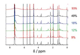
Fig. 2  $^{1}$ H NMR spectra recorded during the RAFT dispersion polymerization of BzMA at 70  $^{\circ}$ C in d<sub>6</sub>-ethanol targeting a final diblock composition of PDMA<sub>43</sub>-PBzMA<sub>500</sub>. Monomer conversions were calculated by comparing the integrals of the vinyl monomer to the t=0 spectrum using TMS as the internal standard.
