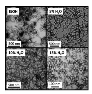
Fig. 6 TEM images of PDMA $_{43}$ -PBzMA $_{120}$  nano objects prepared via RAFT dispersion polymerization of BzMA at 15% w/w in anhydrous ethanol or ethanol/water at 70 °C using AIBN initiator ([PDMA $_{43}$ ]/[AIBN] = 5). The solvent composition is indicated in each case and the morphology varies from a mixed vesicle/worm phase to pure worms to mixed worms/spheres and finally pure spheres as the water content of the continuous phase is increased from 0% to 15% w/w.
