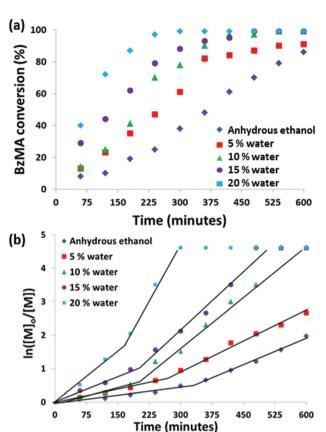
**Fig. 1** Kinetic data derived from  $^1H$  NMR spectroscopy studies for the RAFT dispersion polymerization of benzyl methacrylate (BzMA) at 70 °C using a PDMA $_{43}$  macro-CTA and AIBN initiator ([PDMA]/[AIBN] = 5.0) at 15% w/w solids. The reaction solvent was either anhydrous ethanol or various ethanol/water mixtures with a target composition of PDMA $_{43}$ -PBzMA $_{200}$  in each case. The same data are presented as (a) a conversion-time plot, and (b) a semi-logarithmic plot.
