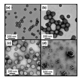
**Fig. 8** TEM images showing the various copolymer morphologies obtained for PDMA<sub>74</sub>–PBzMA<sub>x</sub> diblock copolymer nanoparticles synthesized in 80/20 w/w ethanol/water mixtures; spherical micelles for (a) PDMA<sub>74</sub>–PBzMA<sub>980</sub> (98% BzMA conversion), (b) PDMA<sub>74</sub>–PBzMA<sub>1500</sub> (>99% conversion) and (c) PDMA<sub>74</sub>–PBzMA<sub>1840</sub> (92% conversion) and vesicles for (d) PDMA<sub>74</sub>–PBzMA<sub>2150</sub> (86% conversion).
