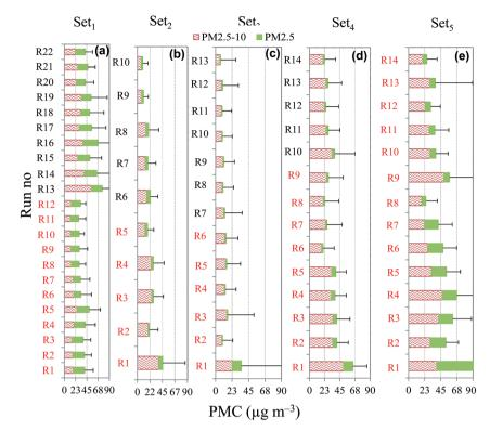
Fig. 2 In-cabin PMCs (PM<sub>2.5-10</sub> and PM<sub>2.5</sub>) in two different fractions during (a) Set<sub>1</sub>, (b) Set<sub>2</sub>, (c) Set<sub>3</sub>, (d) Set<sub>4</sub> and (e) Set<sub>5</sub>. Please note that runs taken during morning hours are marked in red colour. For the sake of clarity only positive standard deviations are shown
