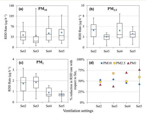
Fig. 6 Average RDD rate of (a)  $PM_{10}$ , (b)  $PM_{2.5}$  and (c)  $PM_1$  during delay conditions at TIs in  $Set_2$ ,  $Set_3$ ,  $Set_4$  and  $Set_5$ . (d) Percentage reduction in incabin RDD rate during different ventilation settings with respect to on-road RDD rate during delay conditions at TIs. Please note that numbers on the x-axis represent the corresponding ventilation setting.
