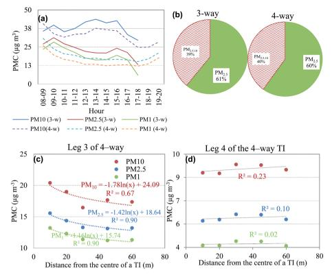
Fig. 4 (a) Diurnal profile of  $PM_{10}$ ,  $PM_{2.5}$  and  $PM_1$  at 3- and 4-way TIs. (b) Percentage contribution of fine and coarse particles to  $PM_{10}$ concentrations at 3- and 4-way TIs. Horizontal profile of PM<sub>10</sub>, PM<sub>2.5</sub> and PM<sub>1</sub> on (c) leg 3 and (d) leg 4 of a 4-way TI.
