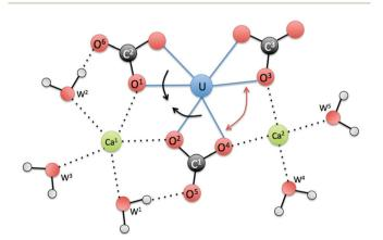
Fig. 7 A schematic view of the equatorial plane around U for the  $Ca_2UO_2(CO_3)_3$  complex in water. W stands for water.
