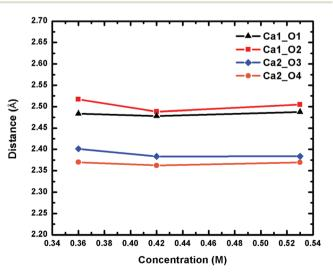
Fig. 4 Change of the four Ca-O<sub>eq</sub> distances of the Ca<sub>2</sub>UO<sub>2</sub>(CO<sub>3</sub>)<sub>3</sub> complex in water at three different concentrations. See Fig. 1 for atom labels. The distances are averages over 15 ps trajectories; the standard deviations for each data point are shown in Fig. S2 of the ESI.†
