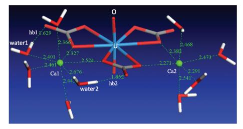
Fig. 6 A snapshot of the  $Ca_2UO_2(CO_3)_3$  complex in water at 0.53 M, showing only the water molecules directly interacting with the two Ca ions; hb1 and hb2 denote hydrogen bonding between the two water molecules (water1 and water2) and the two distal oxygen atoms of the two carbonate groups around Ca1; atom—atom distances are labeled in Å.
